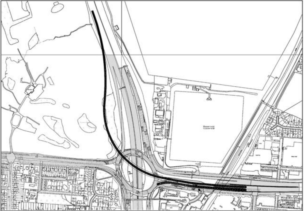
**Figure 4-3 – OPTION 5: A57 to M67 grade separated flyover**
