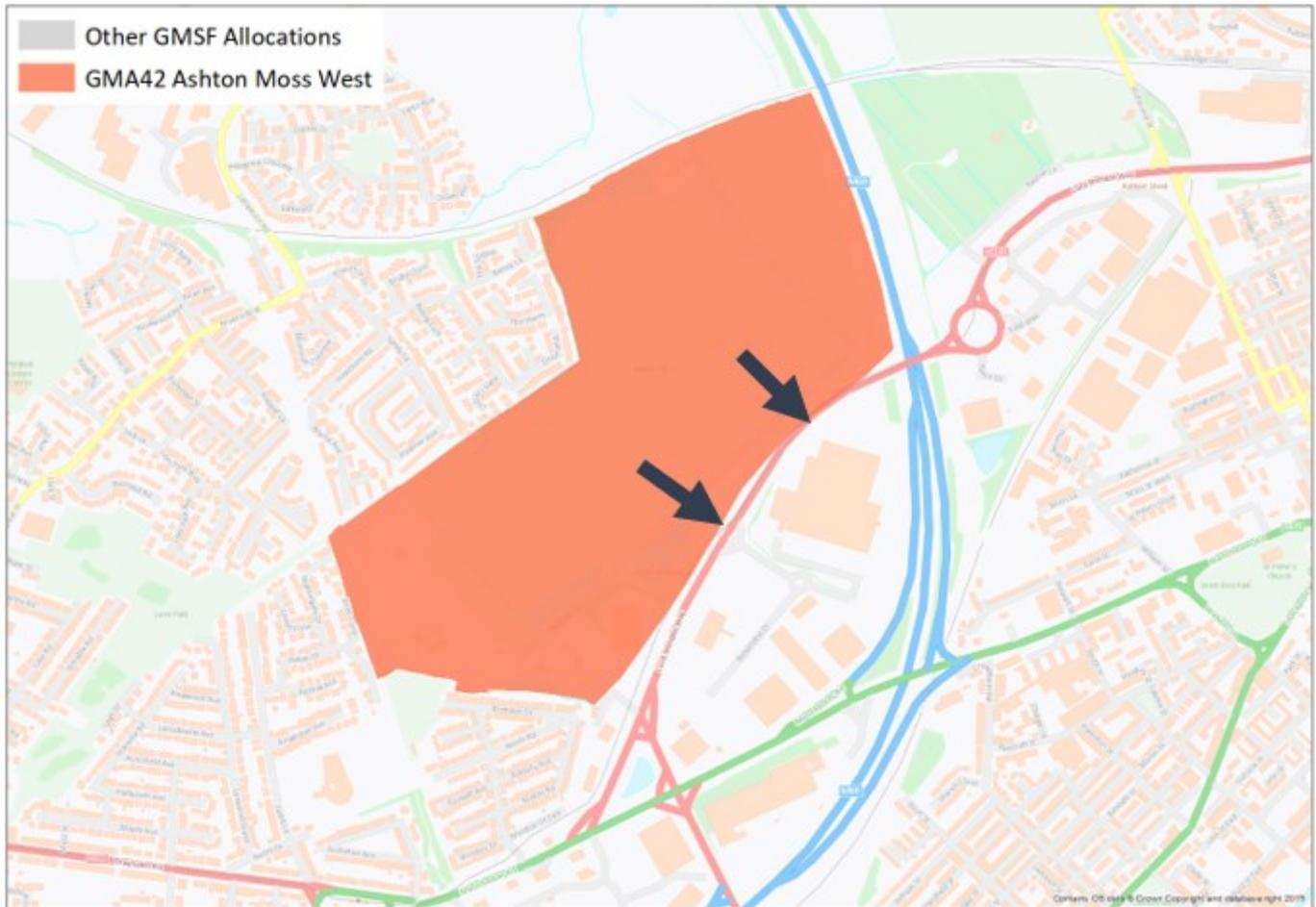
5.1.2 Based on the proposed size of the Ashton Moss West allocation, access would comprise of two primary vehicular accesses directly onto the A6140 Lord Sheldon Way. The main access into the Ashton Moss West allocation would utilise the existing Alexandria Drive access to the Ashton Moss Metrolink P&R facility and Rayner Lane, with the carriageway widths modified to suitably accommodate HGV movements, while also integrating junction facilities for the Ashton Moss P&R and Rayner Lane.
